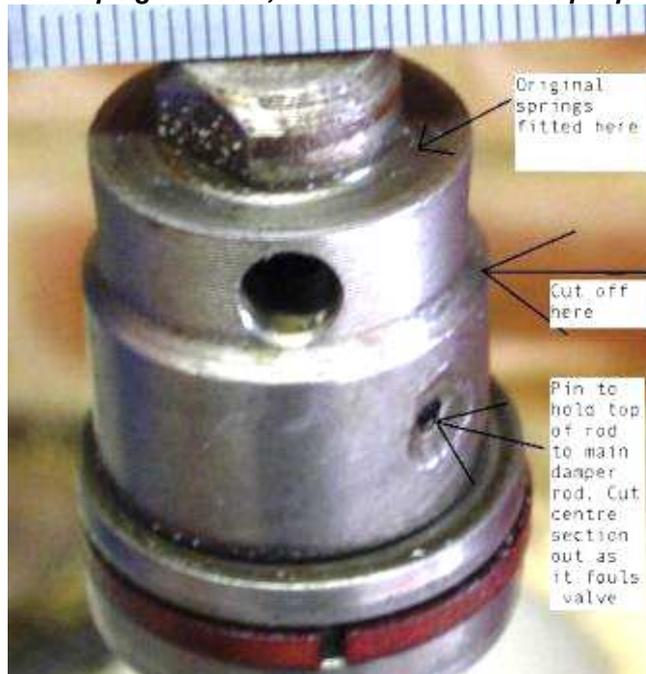
**KYB protruding top style Damping Rod requires machine work along with custom adaptor.**
